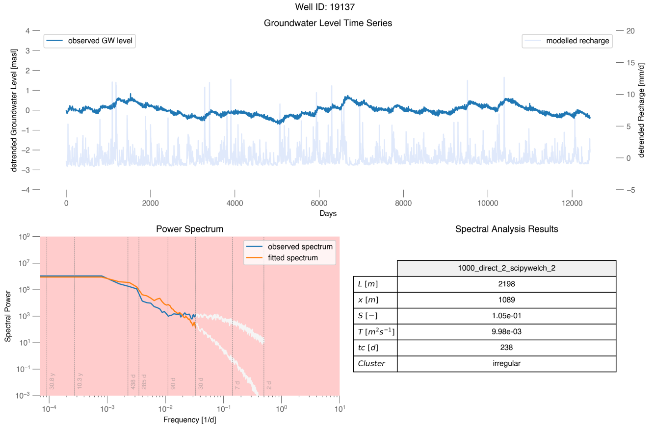
Figure A8. An example of a summary of analysis for a groundwater well of the category irregular . The figure shows the observed groundwater level time series and the modeled mHM recharge Marx et al. (2021), the resulting power spectra for the observed groundwater level and the fitted spectrum with the semi-analytical solution. Only the colored part of the spectrum up to a frequency corresponding to 30 d was taken for the goodness of fit evaluation. The table summarizes the results of the workflow for the selected parameter set. In the presented time series and spectrum, multiple dominant frequencies can be observed: Long-term and multi-annual fluctuations with periods of decades, seasonal fluctuations with a period of a year and short-term fluctuations with periods of weeks to even days. The latter can be most likely attributed to barometric pressure changes in the atmosphere, as variations in summer are less than in winter times. The diverse set of present frequencies in the signal result in a complex shape of the spectrum with several breakpoints. Our simplified semi-analytical approach with a recharge product taken from a land surface model fails to capture the complexity of the processes of this groundwater level fluctuation and was consequently categorized as irregular.
