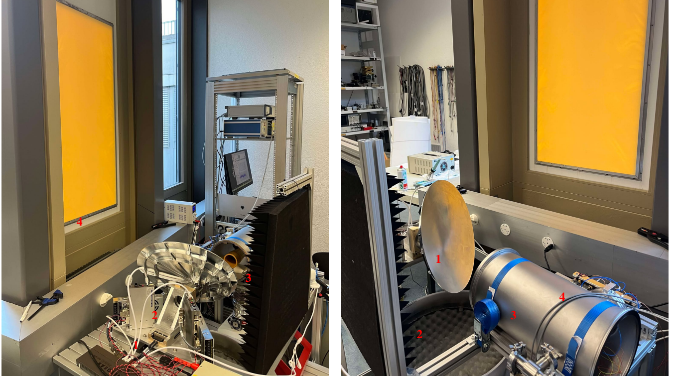
Figure 1. Breadboard assembly of CRYOWARA during first calibration observing the sky at 45^\circ elevation angle. Left panel: 1) Linear stage, 2) Rotating stage, 3) Ambient target, 4) Transparent microwave window, and right panel: 1) Parabolic reflector, 2) LN2 target, 3) Vacuum chamber, 4) front-end chain.
