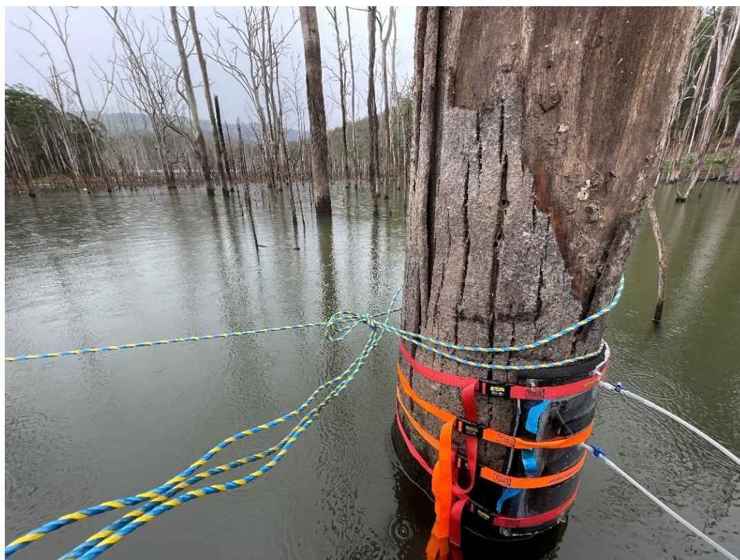
Figure S1: Flux chamber attached against a ghost forest tree at Hinze dam at the lowest measurement on top of Bark.
