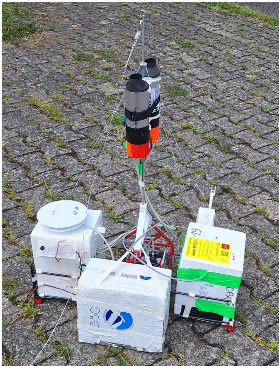
Figure S1. Frontal view of the fully assembled LOONIS Platform. From left to right: the electronics enclosure (containing batteries, pumps, and auxiliary sensors), the POPS unit, and the ozone sonde with an attached radiosonde. The central red frame holds the impactor rack, while a supporting rod extends upward to mount two UCASS instruments.
