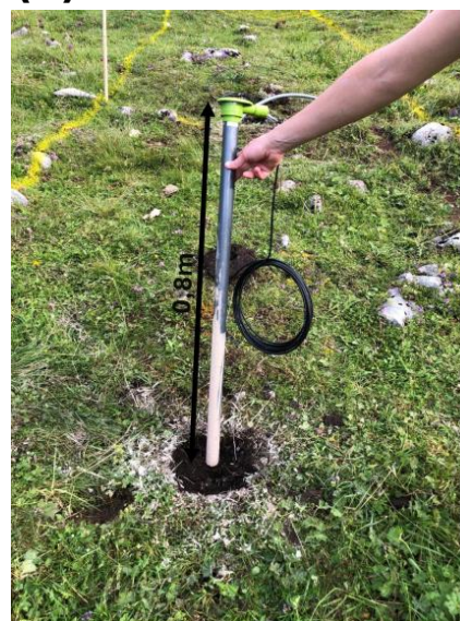
Figure 1. Photographic overview of the large-scale experimental facility. (a) Climate chamber, (b) soil box tilted to 10^\circ with rainfall simulator mounted, (c) macropore pattern plate with rods inserted to visualise the artificial pore network, (d) AquaCheck probes for soil moisture and temperature sensing (as seen in a field application).
