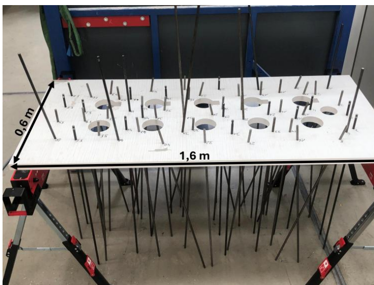
Figure 1. Photographic overview of the large-scale experimental facility. (a) Climate chamber, (b) soil box tilted to 10^\circ with rainfall simulator mounted, (c) macropore pattern plate with rods inserted to visualise the artificial pore network, (d) AquaCheck probes for soil moisture and temperature sensing (as seen in a field application).
