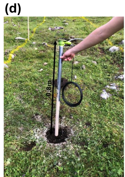
Figure 1. Photographic overview of the large-scale experimental facility. (a) Climate chamber, (b) soil box tilted to 10^\circ with rainfall simulator mounted, (c) macropore pattern plate with rods inserted to visualise the artificial pore network, (d) AquaCheck probes for soil moisture and temperature sensing (as seen in a field application).
