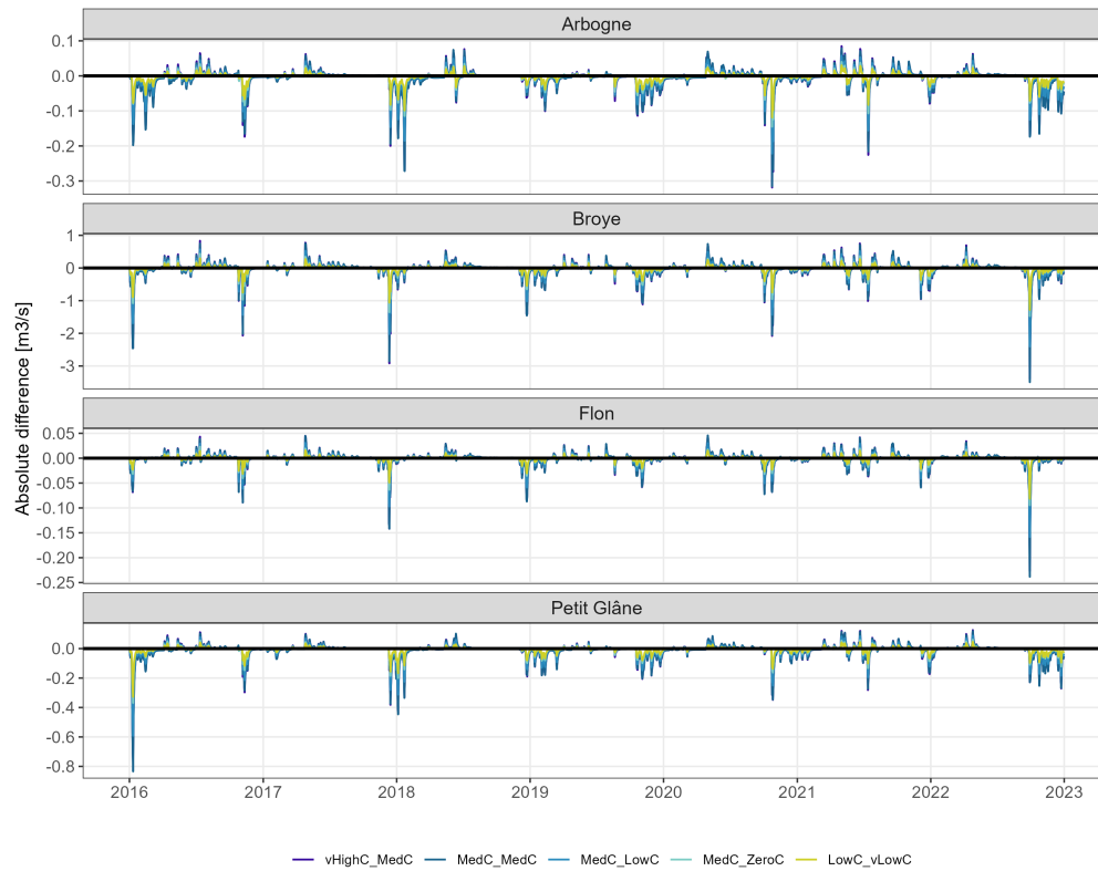
Figure C2. Absolute difference in discharge between the base and each SOC increase scenarios.
