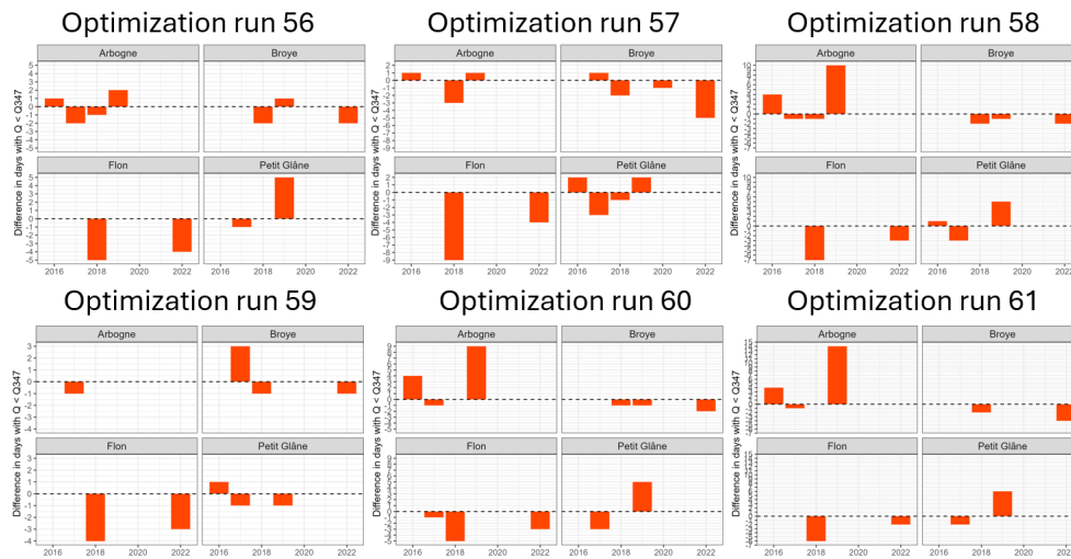
Figure D1. Difference in number of low flow days for base vs. SOC scenario (example scenario MedC_lowC) for 6 different optimization runs with the same settings
