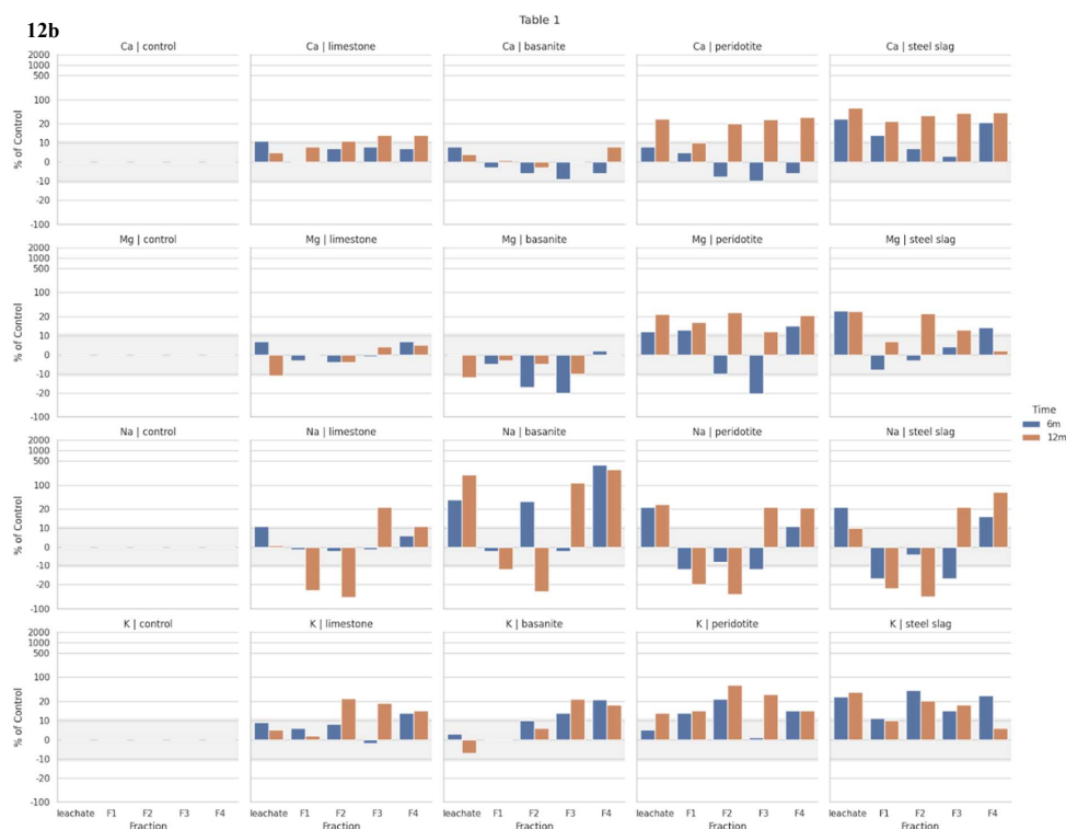
Figure 12: Relative cation partitioning by treatment, time, and pool for acidic LUFA 2.2 B (12a) and slightly alkaline LUFA 6S B (12b). Panels are arranged by ion (rows: \text{Ca}^{2+} , \text{Mg}^{2+} , \text{Na}^+ , \text{K}^+ ) and treatment (columns: control, limestone, basanite, peridotite, steel slag). Within each panel, bars show the percentage of the control for each pool on the x-axis: leachate (cumulative export over the interval) and the four sequential-extraction pools—F1 exchangeable, F2 carbonate-associated, F3 oxide (Fe/Mn-oxide bound), and F4 clay. Colors indicate sampling time (blue = 6 months, orange = 12 months). The y-axis ('% of control') is centered at 0 %; 100 % denotes parity with the control, values >100 % indicate enrichment relative to the control, and <0 % indicates depletion.
