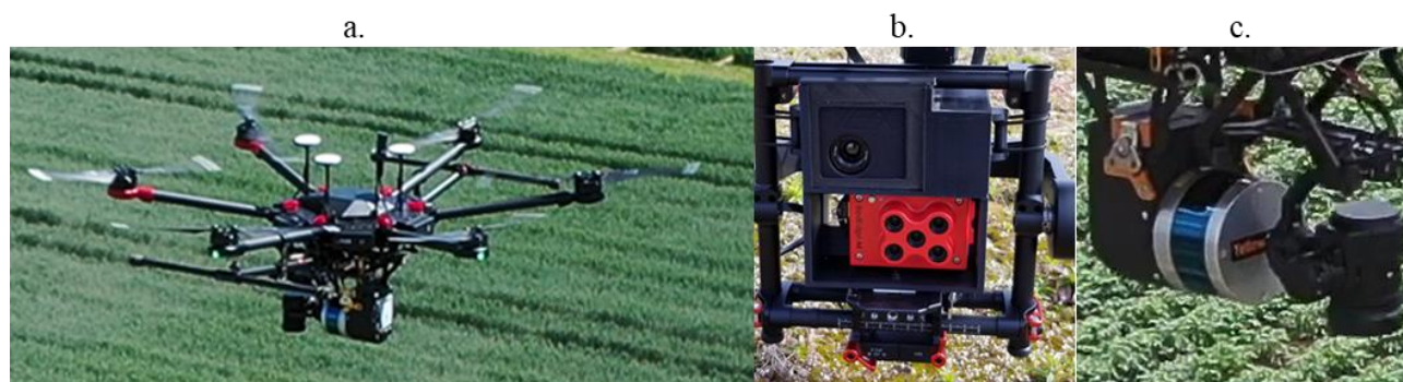
Figure 2: (a.) The DJI Matrice 600 equipped with the YellowScan LiDAR Surveyor and the DJI Zenmuse X1 RGB camera, (b.) the FLIR Vue pro R TIR sensor on top and Micasense RedEdge-M MS sensor on bottom mounted to the DJI Ronin gimbal, and (c.) a closer look at the LiDAR and RGB setup. Note: RGB camera was only used for study area images seen in Figure 1.
