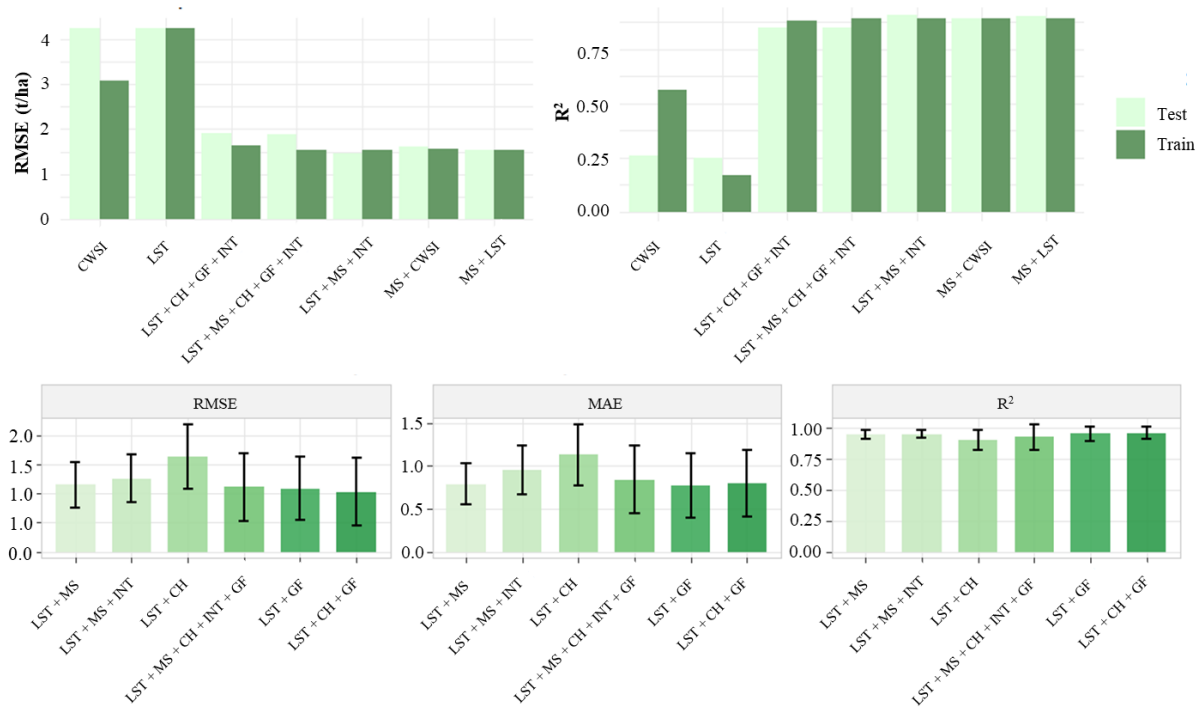
Figure 11: Biomass estimation performance using thermal infrared (TIR) features individually and in combination with multispectral (MS) and LiDAR-derived metrics. Initial comparisons include land surface temperature (LST) and crop water stress index (CWSI) as standalone predictors, after which LST was used for subsequent sensor fusion analyses. LiDAR features include crop height (CH), 5 layer gap fraction (GF), and normalized intensity (INT) using the optimal GF parameterization (20 cm layer
