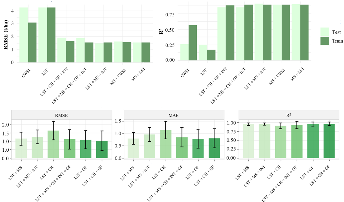
Figure 11: Biomass estimation performance using thermal infrared (TIR) features individually and in combination with multispectral (MS) and LiDAR-derived metrics. Initial comparisons include land surface temperature (LST) and crop water stress index (CWSI) as standalone predictors, after which LST was used for subsequent sensor fusion analyses. LiDAR features include crop height (CH), 5 layer gap fraction (GF), and normalized intensity (INT) using the optimal GF parameterization (20 cm layer depth; 30 cm GSD). Top: 70/30 holdout training and testing performance. Bottom: Repeated stratified 10-fold cross-validation showing mean RMSE, MAE, and R^2 with error bars representing variability among folds.
