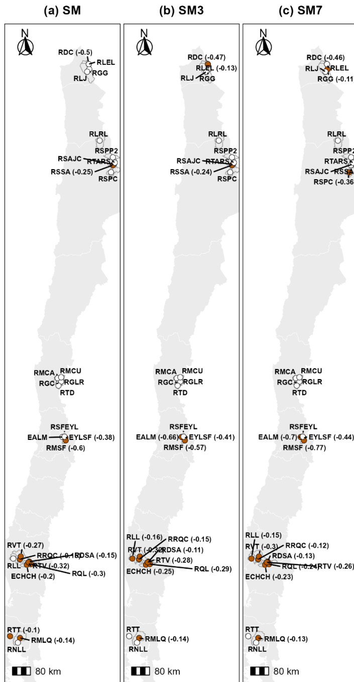
● Positive trend ● Negative trend ○ Not significant trend Figure 4. Trends in soil moisture and its smoothed variants (3-day and 7-day moving averages) for the period 2000–2021. Values in parentheses next to the catchment labels indicate the Theil–Sen slope. The Theil–Sen slope is expressed in units per year: (a) SM in \text{mm yr}^{-1} , (b) SM3 in \text{mm yr}^{-1} , and (c) SM7 in \text{mm yr}^{-1} .
