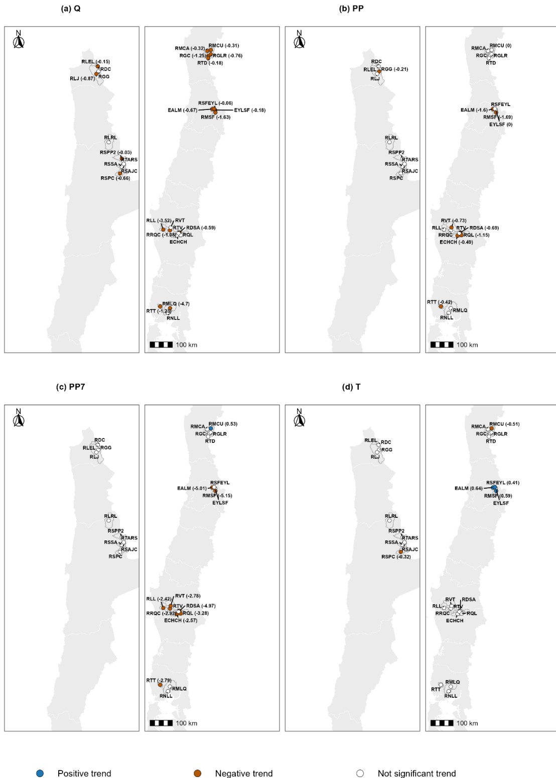
Figure 3. Trends in annual maximum streamflow and associated hydroclimatic variables (precipitation, 7-day accumulated precipitation and temperature) for the period 2000–2021. Values in parentheses next to the catchment labels indicate the Theil–Sen slope. The Theil–Sen slope is expressed in units per year: (a) Q in \text{m}^3 \text{s}^{-1} \text{yr}^{-1} , (b) PP in \text{mm yr}^{-1} , (c) PP7 in \text{mm yr}^{-1} , and (d) T in ^{\circ}\text{C yr}^{-1} .
