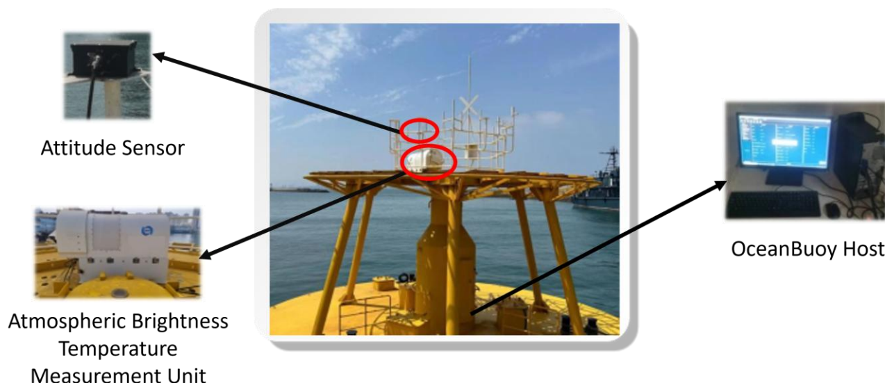
Figure 3: Schematic of the sea trial experimental setup on the 10-meter diameter buoy platform. Key components include: the attitude sensor (top left) for monitoring platform roll and pitch; the QFW-6000 atmospheric brightness temperature measurement unit (bottom left) installed on the upper deck; and the OceanBuoy Host (right) for data aggregation and transmission. The red circles in the central photograph indicate the mounting positions of the sensors on the buoy structure.
