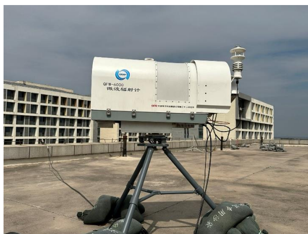
Figure 1: The QFW-6000 microwave radiometric profiler developed by the CETC No.22 Research Institute was deployed for the experiment. The instrument features a K-band and V-band receiver for profiling tropospheric temperature and humidity.
