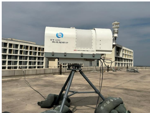
115 Figure 1: The QFW-6000 microwave radiometric profiler developed by the CETC No.22 Research Institute was deployed for the experiment. The instrument features a K-band and V-band receiver for profiling tropospheric temperature and humidity.
