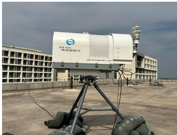
115 Figure 1: The QFW-6000 microwave radiometric profiler developed by the CETC No.22 Research Institute was deployed for the experiment. The instrument features a K-band and V-band receiver for profiling tropospheric temperature and humidity.
