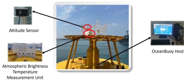
175 Figure 4: Schematic of the sea trial experimental setup on the 10-meter diameter buoy platform. Key components include: the attitude sensor (top left) for monitoring platform roll and pitch; the QFW-6000 atmospheric brightness temperature measurement
