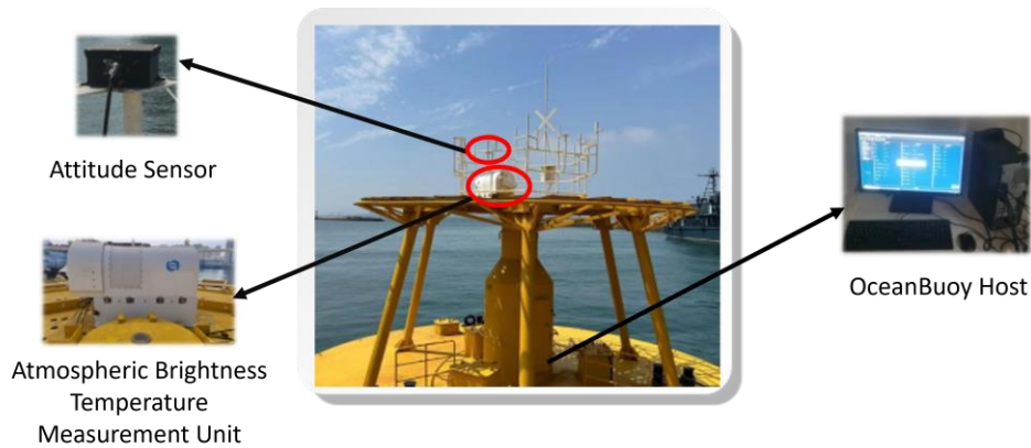
180 Figure 4: Schematic of the sea trial experimental setup on the 10-meter diameter buoy platform. Key components include: the attitude sensor (top left) for monitoring platform roll and pitch; the QFW-6000 atmospheric brightness temperature measurement unit (bottom left) installed on the upper deck; and the OceanBuoy Host (right) for data aggregation and transmission. The red circles in the central photograph indicate the mounting positions of the sensors on the buoy structure.
