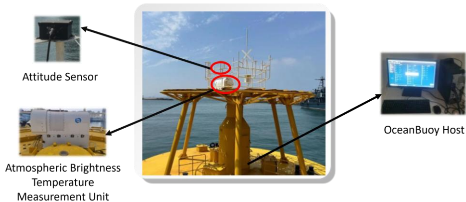
Figure 4: Schematic of the sea trial experimental setup on the 10-meter diameter buoy platform. Key components include: the attitude sensor (top left) for monitoring platform roll and pitch; the QFW-6000 atmospheric brightness temperature measurement unit (bottom left) installed on the upper deck; and the OceanBuoy Host (right) for data aggregation and transmission. The red circles in the central photograph indicate the mounting positions of the sensors on the buoy structure.
