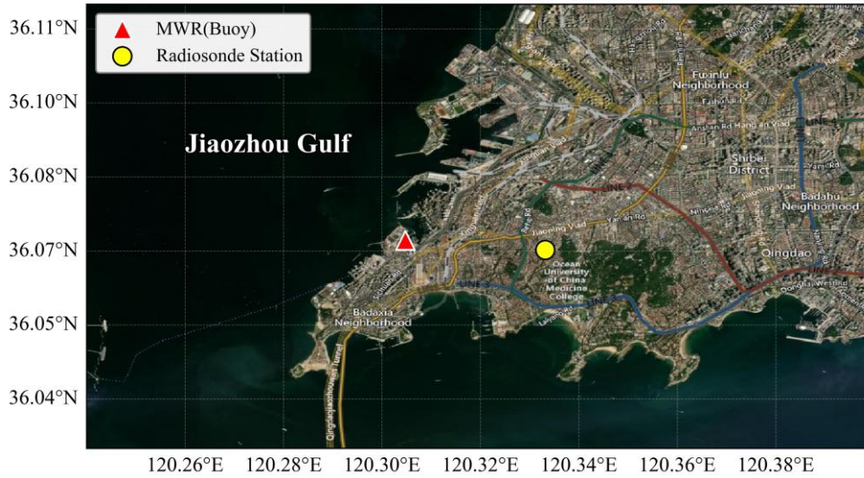
Figure 3: Map of the Jiaozhou Gulf region showing the experimental sites. The red triangle indicates the location of the Buoy-based Microwave Radiometer (36.0721540° N, 120.3047530° E), and the yellow circle represents the Radiosonde Station (36.0702040° N, 120.3331640° E). The two instruments are separated by a distance of approximately 2.5 km. Basemap from Cartopy Quadtree Tiles.
