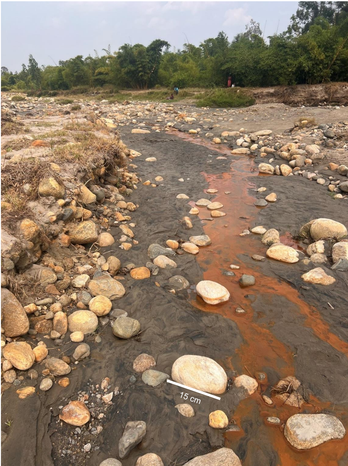
Figure J2: Acid mine drainage from deposited solid tailings at location adjacent to Kasese town, 26 July 2024.
