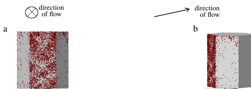
Figure 10. Pattern of 2703 impacted particles distributed over the entire surface of a substrate mount at an initial particle number concentration of 11 \text{ cm}^{-3} corresponding to a total number of about 1.9 \cdot 10^5 particles. Panel a: Frontal view of a substrate mount, panel b: angled side view (Klug, 2024b).
