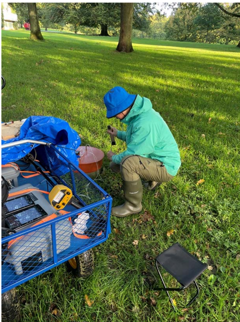
Fig S1: Soil greenhouse gases fluxes measurement with the fast closed chamber approach
