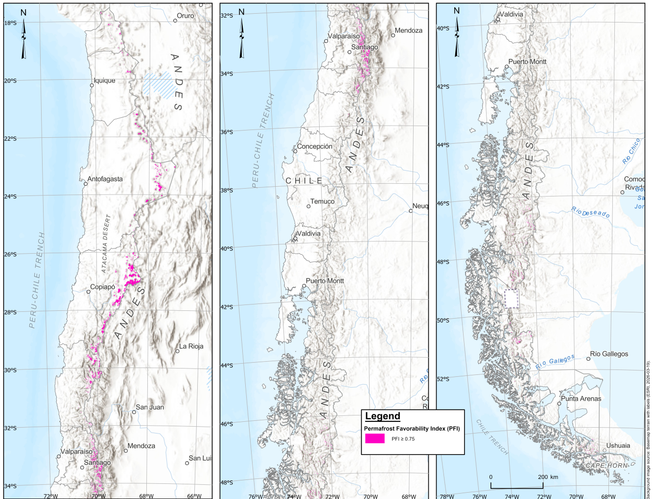
Figure 3. Permafrost favorability map at a 1 km × 1 km resolution, highlighting grid cells containing at least one cell with PFI \geq 0.75 at the full resolution. Basemap Esri Terrain with Labels.
