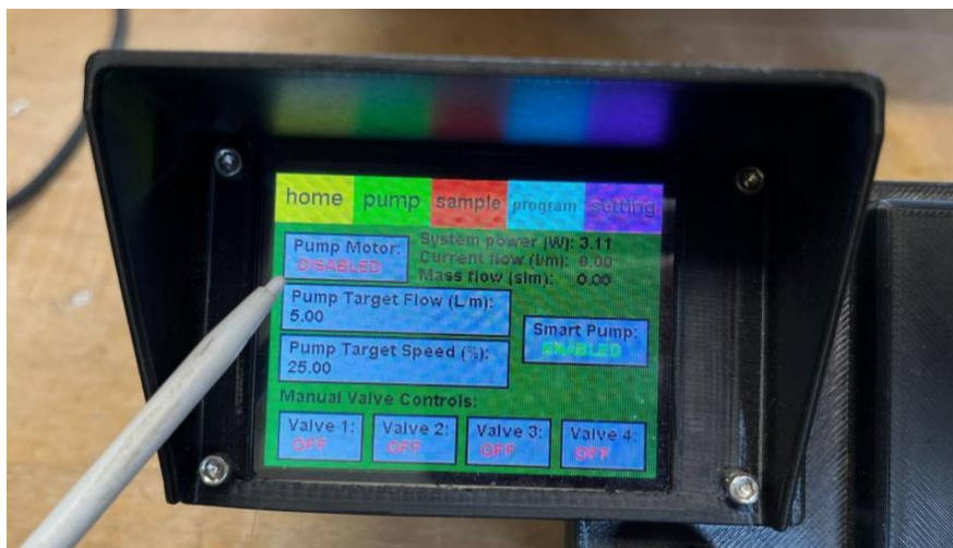
214 Figure 4: Photo of the PUFIN ground station undergoing manual operation. The image depicts the pump motor in an inactive state 215 ('DISABLED') with all four valves closed and 0 sL min -1 of flow. The target flow upon activation is 5.00 sL min -1 .
