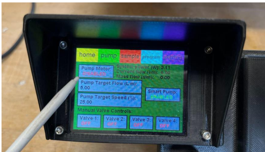
Figure 4: Photo of the PUFIN ground station undergoing manual operation. The image depicts the pump motor in an inactive state ('DISABLED') with all four valves closed and 0 sL min -1 of flow. The target flow upon activation is 5.00 sL min -1 .
