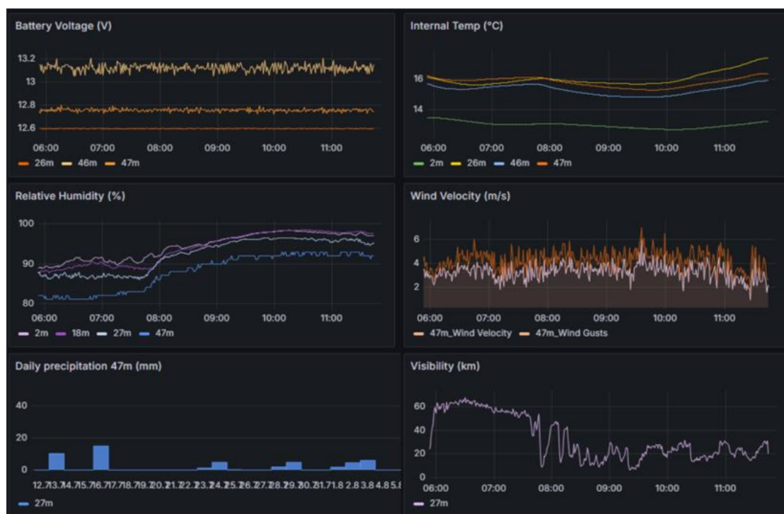
Figure 5: Screenshot of Grafana dashboard showing data from weather stations installed on above-canopy tower.
