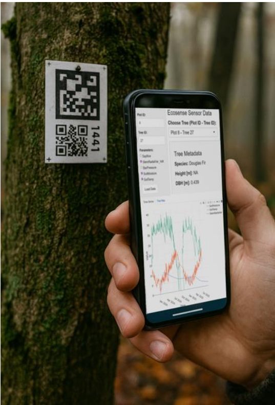
Figure 8: Field access to tree-level data streams. Scanning a QR-coded tag on a tree launches the ECOSENSE Shiny app on a smartphone, retrieving the associated tree information, such as time series from the central database.
