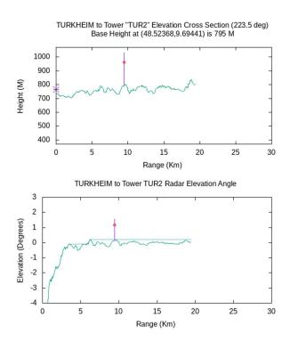
Cross section from radar TUR to turbine "TUR2". Top: topographic height ASL. Bottom: radar elevation angle of topography assuming 30m antenna height. In elevation image the flat lines extend from lowest elevation visible to next visible topography,
