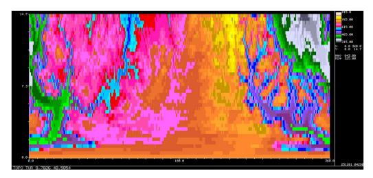
Coarse view of topography around TUR radar; SRTM30 data (~90m) as B-scan. Yellows are heights above 765m, which 735m ASL ground level at TUR radar plus assumed 30m antenna height. (Relates to Figure 3.)
