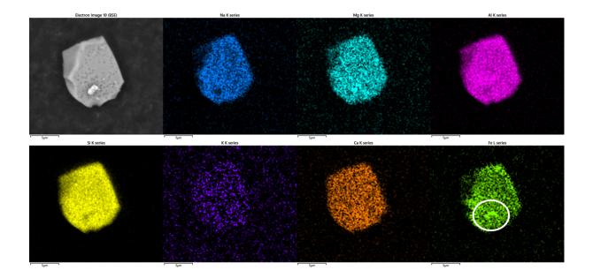
SEM image and corresponding energy dispersive X-ray spectroscopy (EDX) elemental maps of Sodium (Na), Magnesium (Mg), Aluminum (Al), Silicon (Si), Potassium (K), Calcium (Ca), and Iron (Fe) on representative "MAS" particle. Increased brightness indicates more of the element. The white circles emphasize the Fe-rich inclusions.
