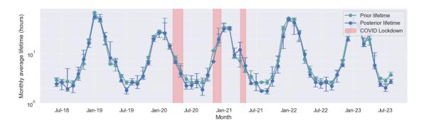
The reported improved performance is based on using the domain average lifetime of the simulation as the prior for the inversion. When applying to measured TROPOMI data, the prior lifetime is estimated from the average OH concentration in CAMS. However, a domain average lifetime is a poor approximation to a lifetime that is an explicit non-linear function of NO2.
