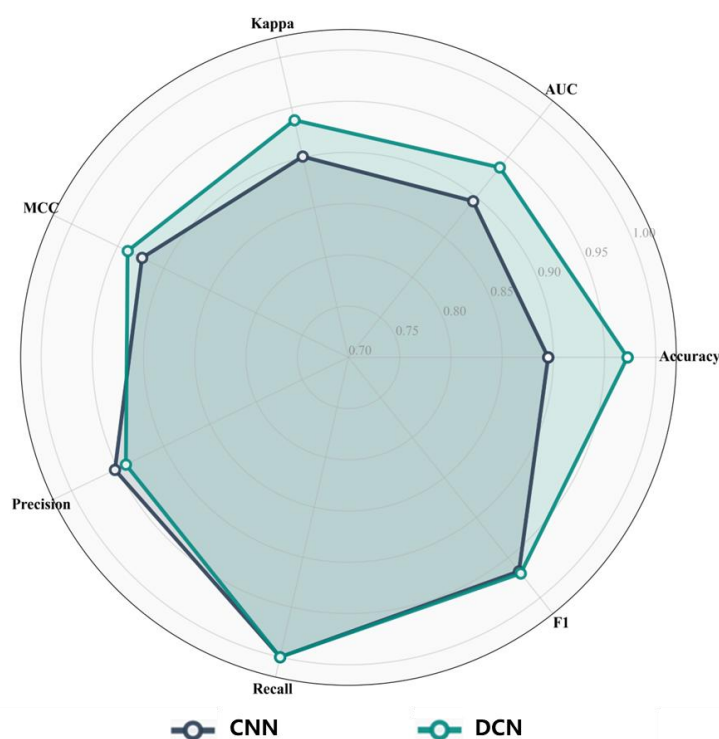
450 Figure 12: Evaluation of model performance between CNN and DCN in Accuracy, Precision, Recall, F1-score, AUC, Kappa, and MCC.
