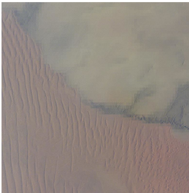
Figure 4. Nadir top of atmosphere (TOA) view of the Gobabeb HYPERNETS site in Namibia (De Vis et al., 2024) with a plane-parallel atmosphere (AFGL 1986 US Standard profile, no aerosols). The surface shape is a triangulation of the Copernicus GLO-30 DEM (30 m resolution) with a diffuse reflection model textured by a resampling at 1 km of the HAMSTER dataset (Roccetti et al., 2024).
