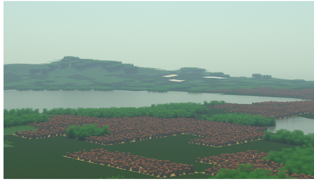
Figure 5. RGB view of a synthetic scene created after the area of Mbita, on Lake Victoria in Kenya. The surface shape (a triangulation of the Copernicus GLO-30 DEM) is assigned different reflection models ( e.g. water, diffuse, RPV) based on land cover information contained in a texture encoded as a PNG image. Where relevant, land areas are also tiled with 3D objects at a reduced memory cost using instancing: a few templates ( e.g. village, forest) are cloned many times to create a radiatively plausible reflection pattern. See also Section 8.2.3 for a similar example.
