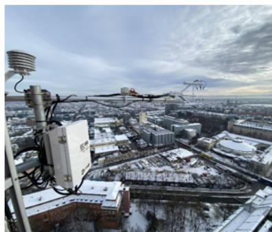
Figure C1. Photos of the measurement sites in Zurich, Paris, and Munich. The black arrows indicate the height at which the IRGASON and the gas inlets (two REA inlets with fast-response valves for updrafts and downdrafts, one inlet for REA quality control tests, one inlet for MGA 7 measurements) were mounted. Pictures from Pekka Pelkonen (ICOS RI), Pedro Henrique Herig Coimbra (INRAE), and Reiter Antennenbau-Energietechnik GmbH.
