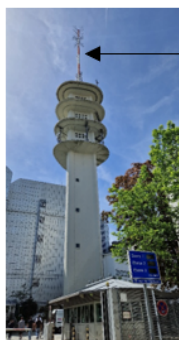
Figure C1. Photos of the measurement sites in Zurich, Paris, and Munich. The black arrows indicate the height at which the IRGASON and the gas inlets (two REA inlets with fast-response valves for updrafts and downdrafts, one inlet for REA quality control tests, one inlet for MGA 7 measurements) were mounted. Pictures from Roland Vogt (University of Basel) , Pekka Pelkonen (ICOS RI), Pedro Henrique Herig Coimbra (INRAE), and Reiter Antennenbau-Energietechnik GmbH.
