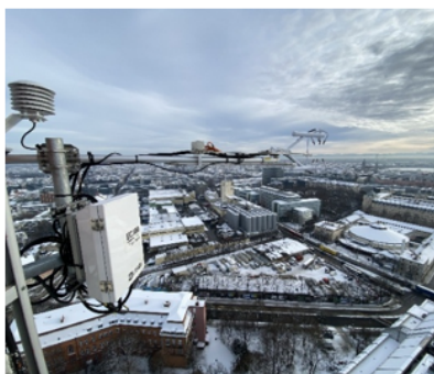
Figure C1. Photos of the measurement sites in Zurich, Paris, and Munich. The black arrows indicate the height at which the IRGASON and the gas inlets (two REA inlets with fast-response valves for updrafts and downdrafts, one inlet for REA quality control tests, one inlet for MGA 7 measurements) were mounted. Pictures from Roland Vogt (University of Basel) , Pekka Pelkonen (ICOS RI), Pedro Henrique Herig Coimbra (INRAE), and Reiter Antennenbau-Energietechnik GmbH.
