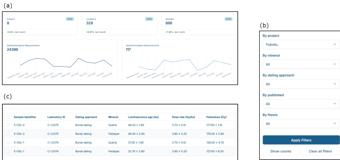
Figure 3. An example of the user interface implemented with Django Unfold that show (a) an overview of all available measurements from different projects that are stored in the database, grouped in sedimentological and geochronological measurements, (b) the filtering feature to extract specific data from the data base and (c) the resulting data from the query, in this case geochronological data from the Toboliu project.
