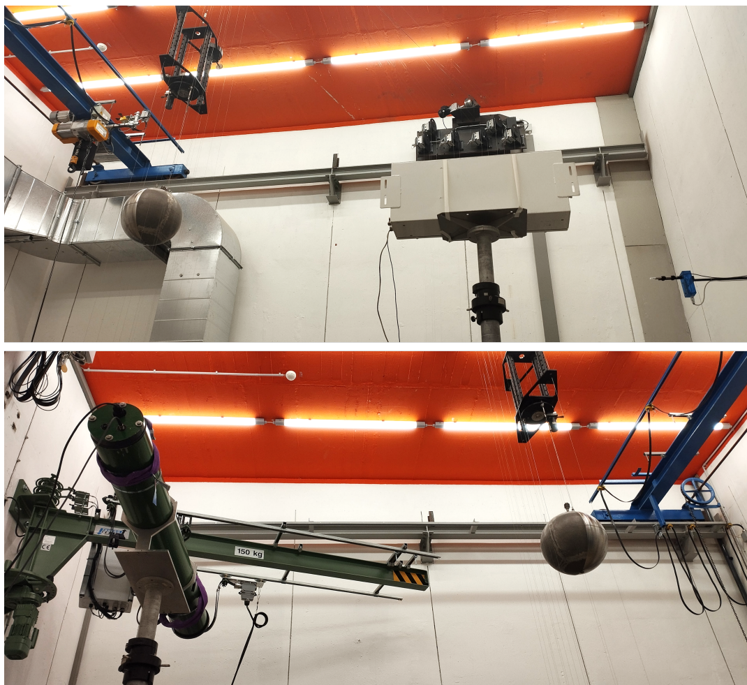
Figure 7. CRS1000 (top) and System S1 (bottom) in the PTB irradiation room during irradiation with the moderated ^{252}\text{Cf} source. The moderator sphere, with the Cd foil facing the detector, is also visible in both images.
