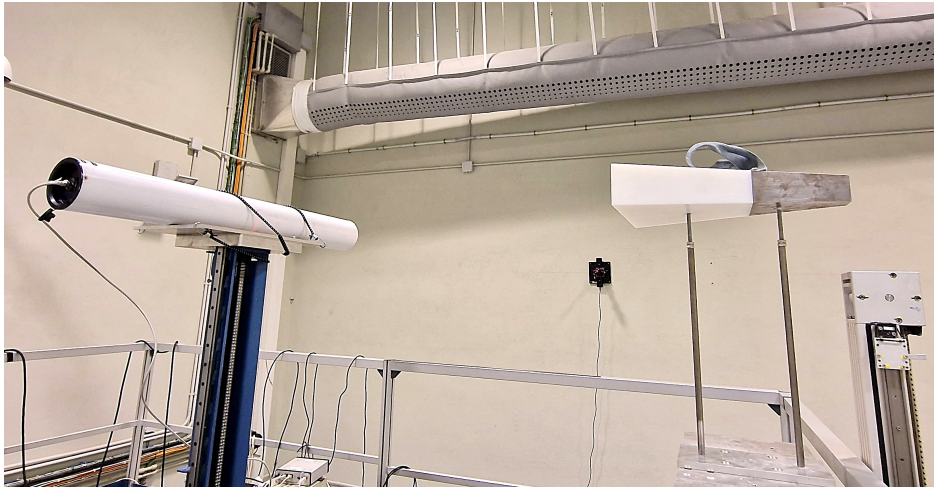
Figure 9. Irradiation at CIEMAT of one of the CRS2000/B tubes with the shadow object with pyramidal geometry, kindly provided by the Universidad Politécnica de Madrid (UPM).
