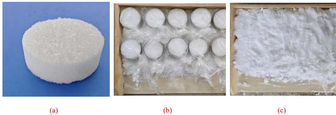
Figure 1: Sample preparation process ((a) Compacted specimen; (b) Samples covered with membranes; (c) Sprinkling snowflakes).
