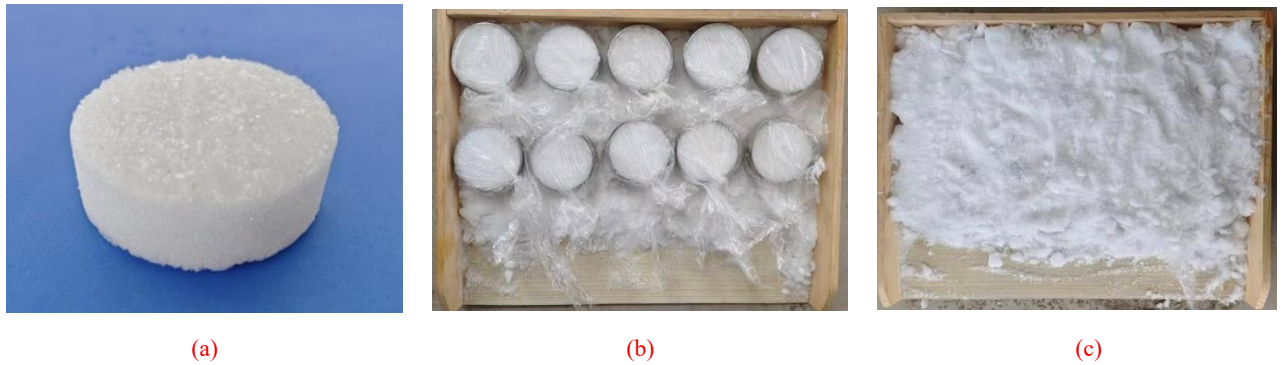
Figure 1: Sample preparation process ((a) Compacted specimen; (b) Samples covered with membranes; (c) Sprinkling snowflakes).
