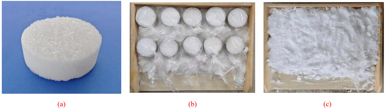
470 Figure 1: Sample preparation process ((a) Compacted specimen; (b) Samples covered with membranes; (c) Sprinkling snowflakes).
