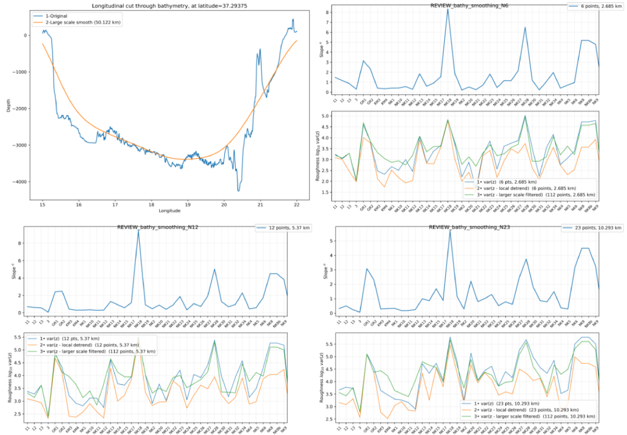
Fig. R3. Setup of the bathymetric smoothing applied to the GEBCO product. The first panel shows the smoothed bathymetry together with a longitudinal section across the Ionian Basin at the mid-latitudes of the study area. The other panels display the slope and roughness computed using spatial windows of 6 points (2.7 km), 12 points (5.3 km), and 23 points (10.3 km). Roughness is estimated using three approaches: (1•) the variance of bathymetry within the window (our current method), (2•) the variance of bathymetry after removing a local smoothing within the window, and (3•) the variance of bathymetry after removing the large-scale smoothing.
