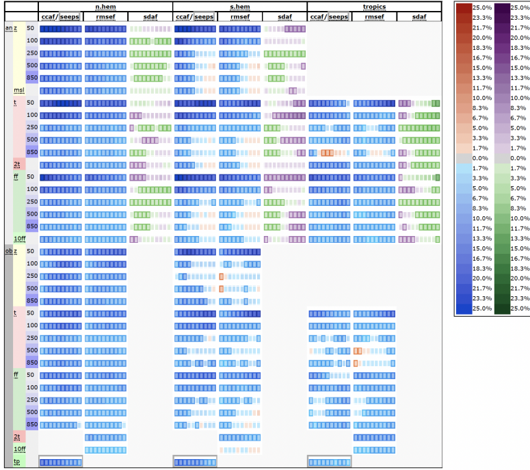
Figure 7: Scorecard comparing forecast scores of AIFS revised versus the previous AIFS version for the whole year of 2023. Forecasts are initialised on 00 and 12 UTC. Relative score changes are shown as function of lead time (day 1 to 10) for northern extra-tropics (n.hem), southern extra-tropics (s.hem) and tropics. Blue colours mark score improvements and red colours score degradations. Purple colours indicate an increased in standard deviation of forecast anomaly, while green colours indicate a reduction. Framed rectangles indicate 95% significance level. Numbers behind variable abbreviations indicate variables on pressure levels (e.g., 500 hPa), and suffix indicates verification against IFS NWP analyses (an) or radiosonde and SYNOP observations (ob). Scores shown are anomaly correlation (ccaf), SEEPS (seeps, for 24h precipitation accumulation), RMSE (rmsef) and standard deviation of forecast anomaly (sdaf).
