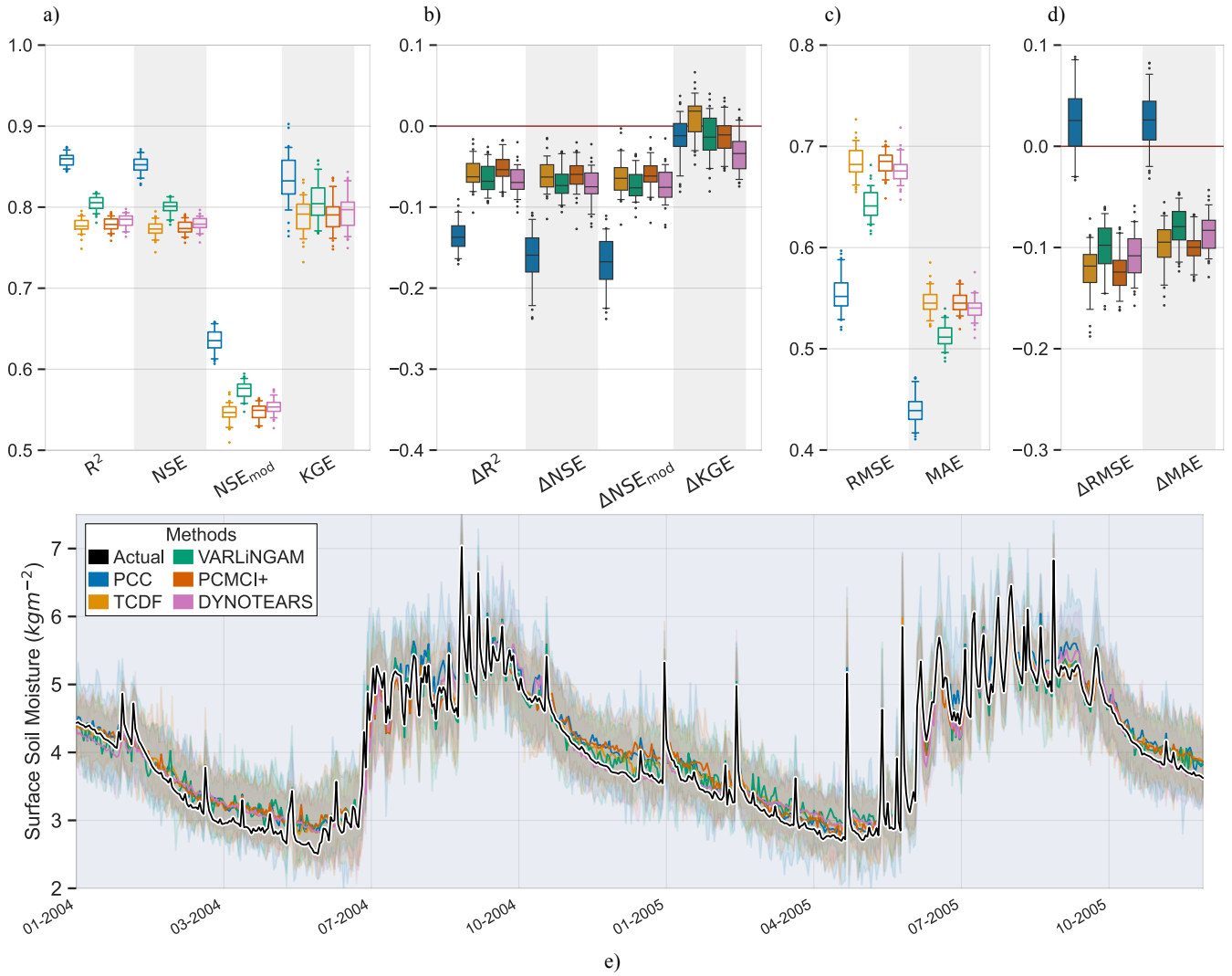
Figure 7. Performance and error metrics of the machine learning models created for surface soil moisture prediction. Panels a) and c) show the performance and error metrics during the training period. While panels b) and d) show the difference in performance and error metrics between the testing and training, eg: \Delta R^2 = R^2_{testing} - R^2_{training} . Panel e) shows the predicted and actual time-series in the testing period, based on PCC and CD-based models. For each method, the plot shows the mean prediction of the 100 Monte Carlo simulations, while the shading shows the minimum and maximum range. The metrics adopted are commonly used metrics in hydrology. R^2 -Coefficient of Determination, NSE -Nash-Sutcliffe efficiency, NSE_{mod} -modified Nash-Sutcliffe efficiency, KGE -Kling-Gupta efficiency, RMSE -Root Mean Square Error and MSE -Mean Squared Error, Jackson et al. (2019). (A \Delta(\cdot) < 0 for performance metrics means a drop in performance during the testing period compared to the training period. While a \Delta(\cdot) > 0 for error metrics means a drop in performance during the testing period compared to the training period.)
