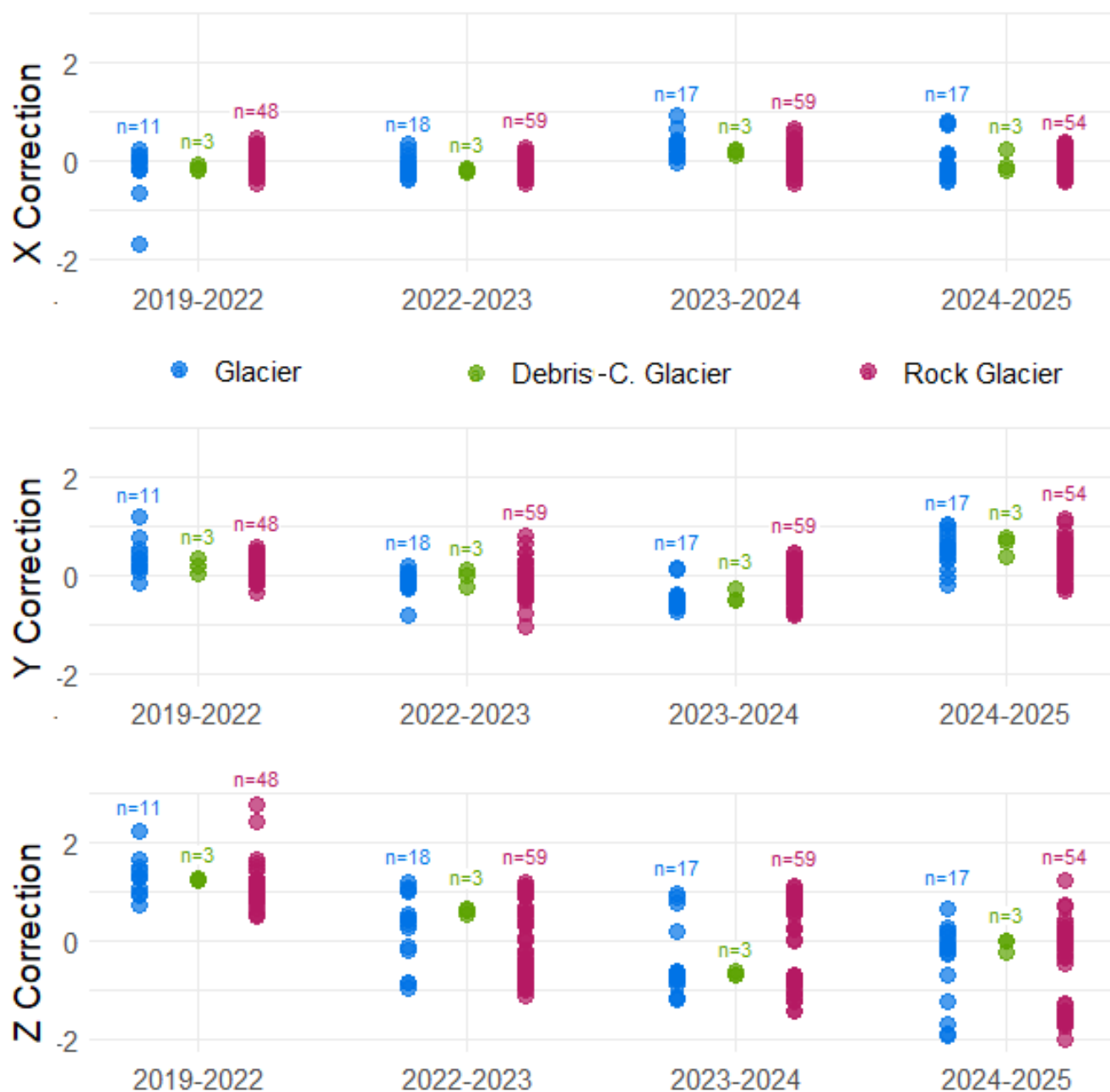
Fig. S2 Temporal and landform-specific analysis of the x, y and z correction factors (m) used during co-registration. For a full list of all correction factors, please see A3. Co-registration is achieved following the approach by Nuth and Kääb (2011) as applied in Demcoreg (Shean et al. 2016). The number of landforms in the respective category is given in each of the subplots and depends on the respective acquisition extents, see A1.
