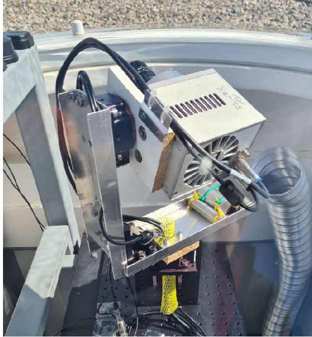
Figure 1 Photo of the scanning FAIM instrument. The azimuth rotation stage is below the horizontal metal frame, the second stage is vertically oriented to provide the possibility to rotate the camera to different zenith angles. The construction is counterweighted to prevent for unilateral strain and provide a longer lifetime of the mechanical components. The instrument is located below an air-ventilated acrylic dome at Oberpfaffenhofen.
