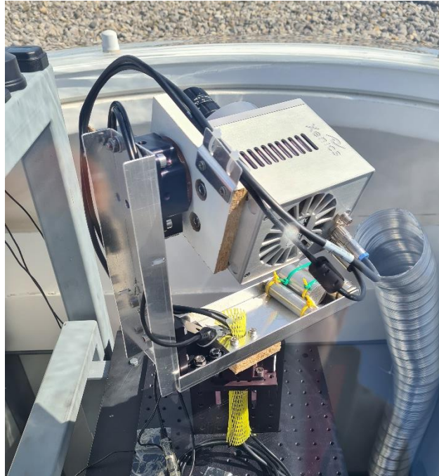
105 Figure 1 Photo of the scanning FAIM instrument. The azimuth rotation stage is below the horizontal metal frame, the second stage is vertically oriented to provide the possibility to rotate the camera to different zenith angles. The construction is counterweighted to prevent for unilateral strain and provide a longer lifetime of the mechanical components. The instrument is located below an air-ventilated acrylic dome at Oberpfaffenhofen.
