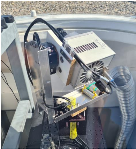
110 Figure 1 Photo of the scanning FAIM instrument. The azimuth rotation stage is below the horizontal metal frame, the second stage is vertically oriented to provide the possibility to rotate the camera to different zenith angles. The construction is counterweighted to prevent for unilateral strain and provide a longer lifetime of the mechanical components. The instrument is located below an air-ventilated acrylic dome at Oberpfaffenhofen.
