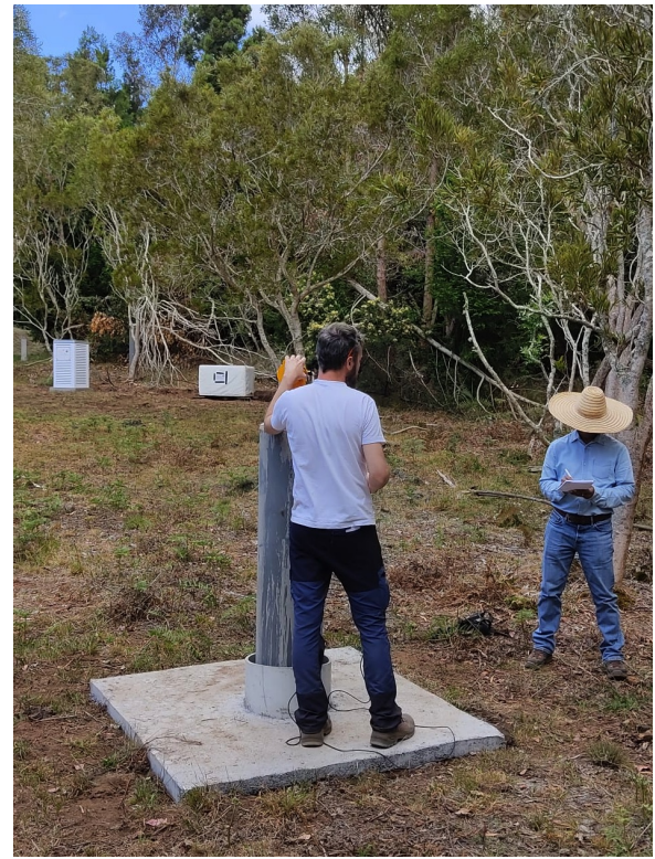
Figure 2. Left: a schematic map of the observatory. Right: Photograph showing the layout of the La Réunion Observatory. In the foreground, the main observatory pillar is seen during a training session. In the background, from left to right, are: the grey concrete target pole; the white meteorological box housing the sensor electronics; the grey vertical PVC tube, partially obscured by trees, containing the variation scalar magnetometer; and the plastic box containing the variation vector magnetometer, covered with a white thermal blanket.
