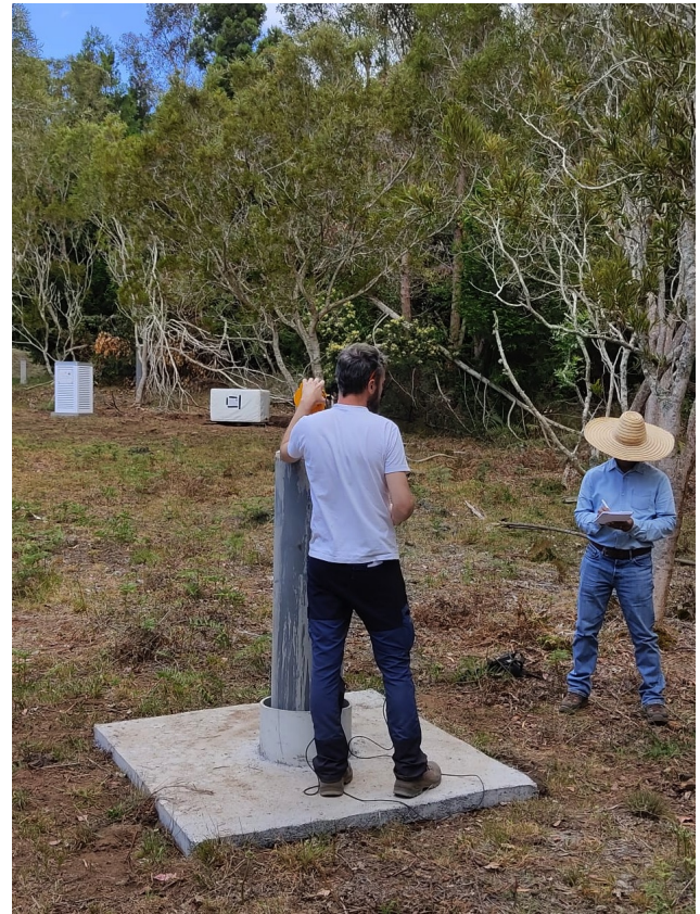
Figure 2. Left: a schematic map of the observatory. Right: Photograph showing the layout of the La Réunion Observatory. In the foreground, the main observatory pillar is seen during a training session. In the background, from left to right, are: the grey concrete target pole; the white meteorological box housing the sensor electronics; the grey vertical PVC tube, partially obscured by trees, containing the variation scalar magnetometer; and the plastic box containing the variation vector magnetometer, covered with a white thermal blanket. Picture showing the layout of the La Réunion observatory. In front, the absolute pillar during a training session with in the background, from left to right, the grey concrete target pole with the azimuth target attached, the meteorology type white box containing the sensors electronics, the grey vertical PVC tube partly hidden behind the trees containing the variation scalar magnetometer and the plastic box containing the variation vector magnetometer, covered with a thermal white blanket.
